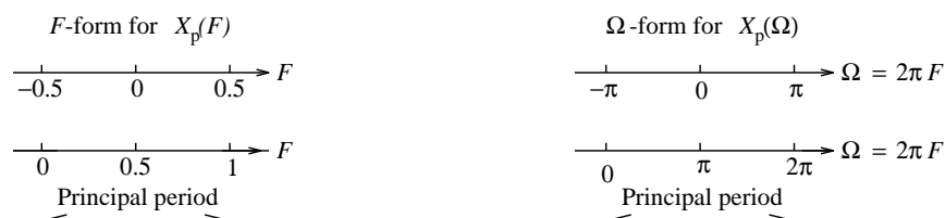
Figure 5.2 Various ways of plotting the DTFT spectrum
